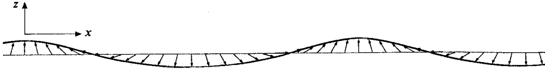
FIGURE 1. Sketch of an initially horizontal material contour and the associated displacement field \xi(x, t) in a deep-water wave, for one value of z and a number of equally spaced values of x . The horizontal line marks the given value of z . By (6), the latter gives the mean depth of the set of material particles located at the tips of the displacement arrows (i.e. at positions x + \xi ). Note that, because the average is evenly weighted over x rather than x + \xi , the horizontal line lies higher than a line cutting off equal areas.
