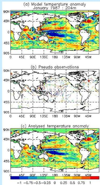
**Figure 1:** Reconstruction (c) of model temperature anomalies (a) at 204m by optimal interpolation of 'pseudo observations' (b) sampled at typical real world observation density.
